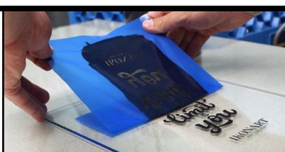
**APPLICATION OF PAINT OR INK** Apply paint or ink to surface. Squeegee or brush to cover all open areas of the stencil. Depending on your substrate, you can squeegee the surface to remove excess paint or ink. Carefully remove the IKONART stencil. Let substrate dry completely.
