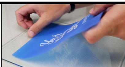
**APPLICATION OF IKONART TO SUBSTRATE** Place a mark on the carrier sheet (shiny side) of the IKONART stencil indicating the back (after use, stencil must be reapplied to the same side of the carrier sheet that it was removed from). Remove the carrier sheet (do not throw away). Place IKONART stencil, adhesive side down, on substrate and apply light pressure to remove bubbles.
